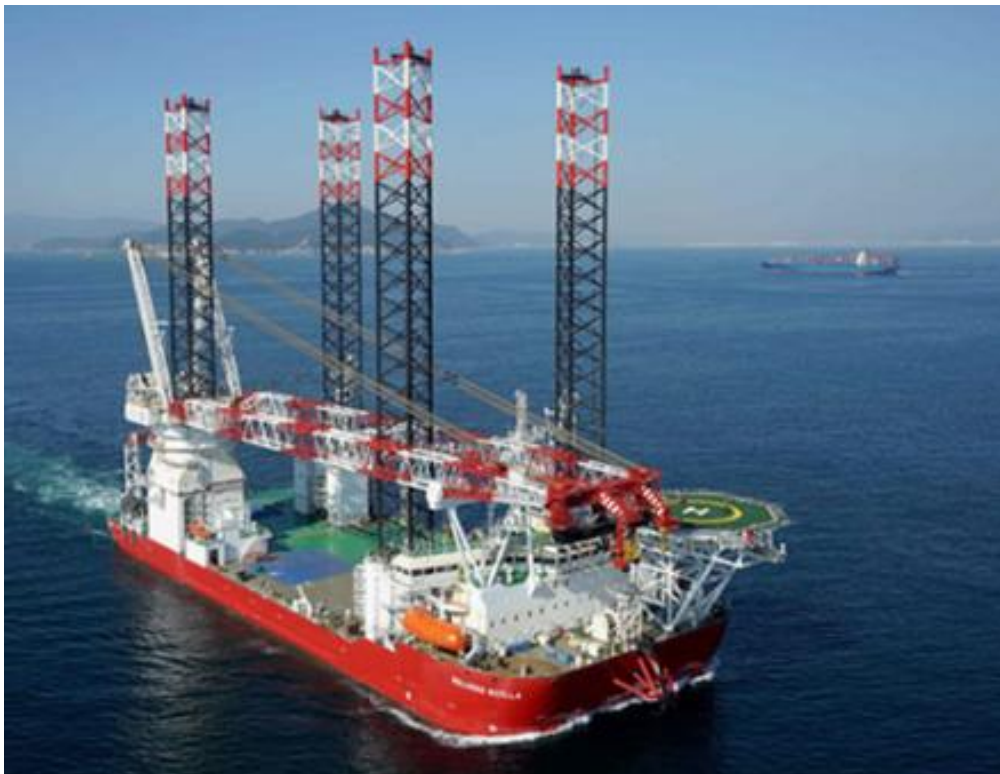
Figure 9. Jacket installation Vessel.
