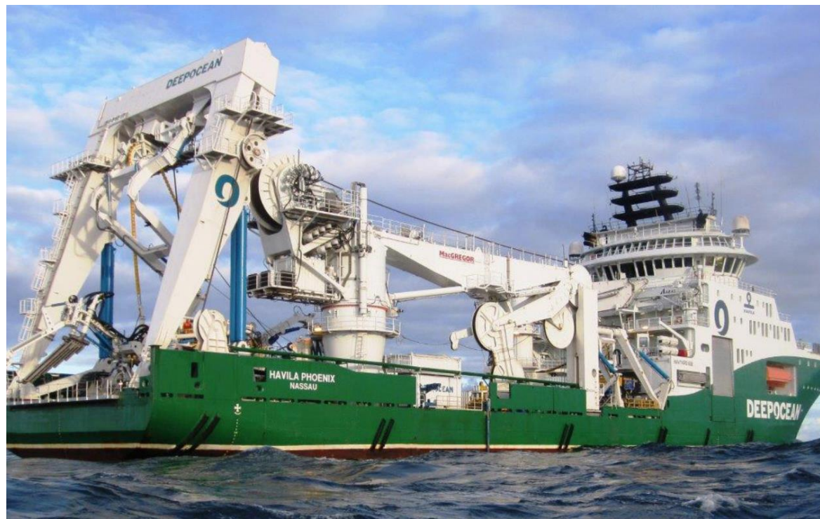
Figure 16. Cable burial vessel.
