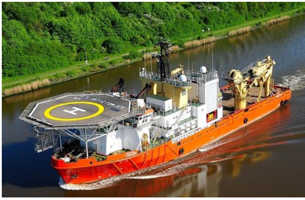
Figure 5 Boulder Picking Vessel
