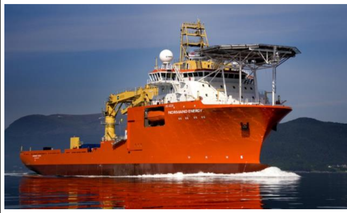
Figure 4. Soil Plug Removal Vessel
