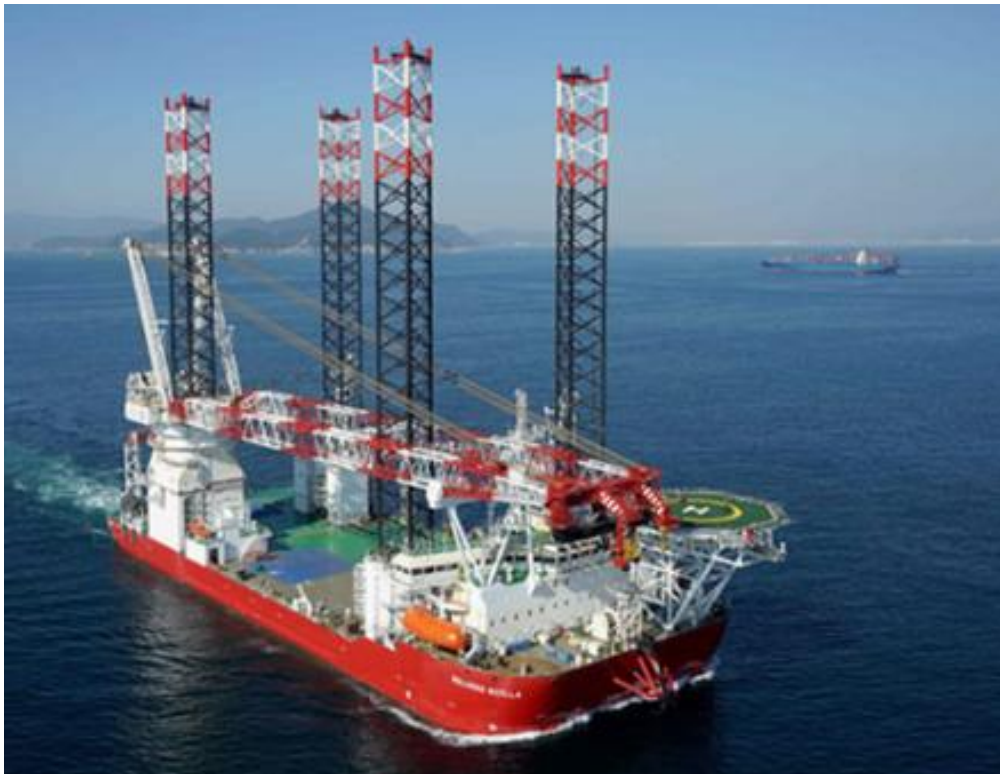
Figure 9. Jacket installation Vessel.
