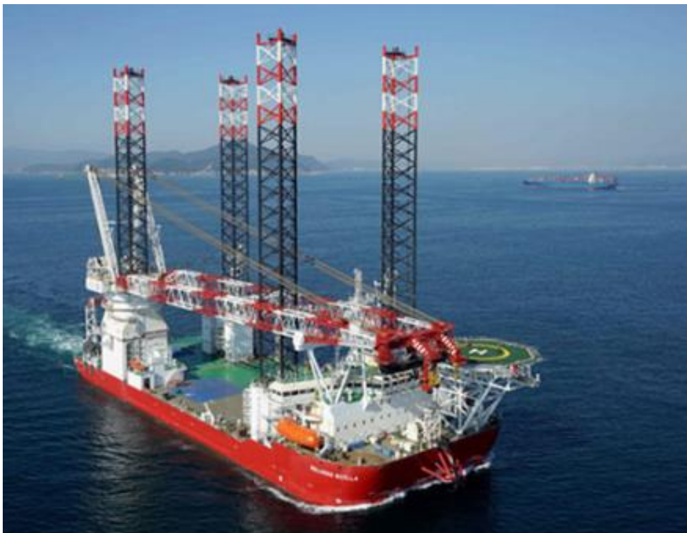
Figure 9. Jacket installation Vessel.
