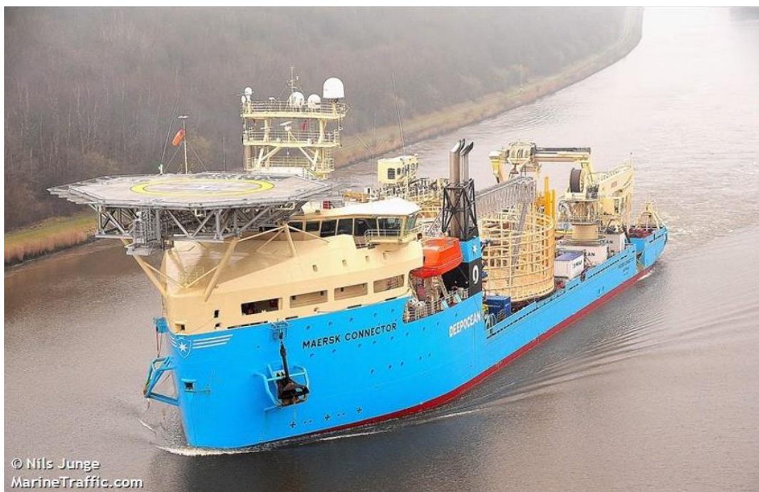
Figure 22. Rock Bag Placement and Boulder clearance vessel
