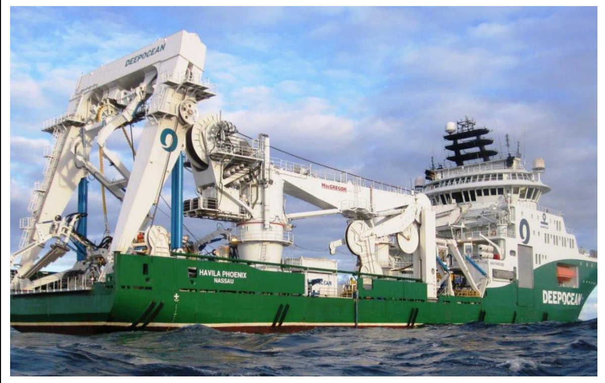
Figure 15. Cable burial vessel.
