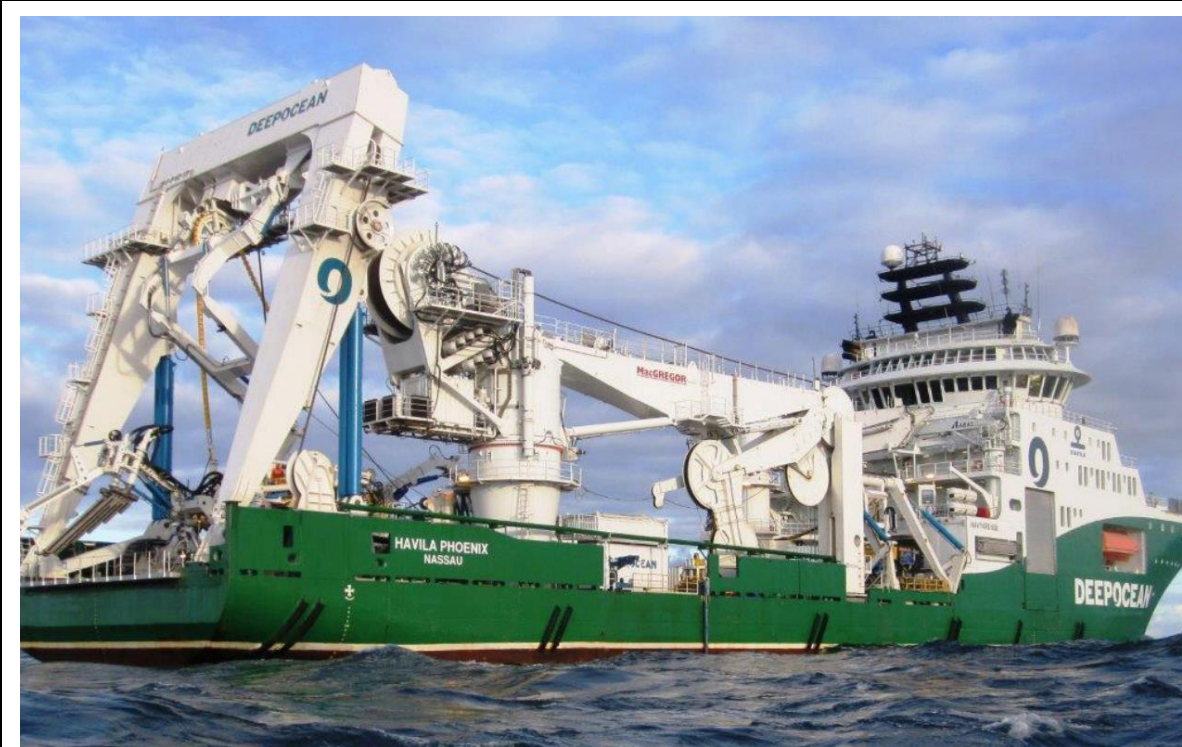
Figure 15. Cable burial vessel.
