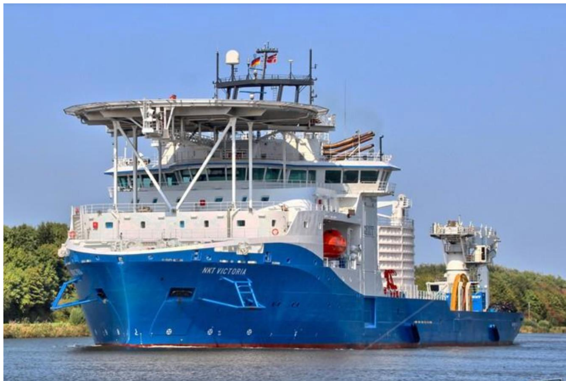
Figure 15. Cable lay vessel
