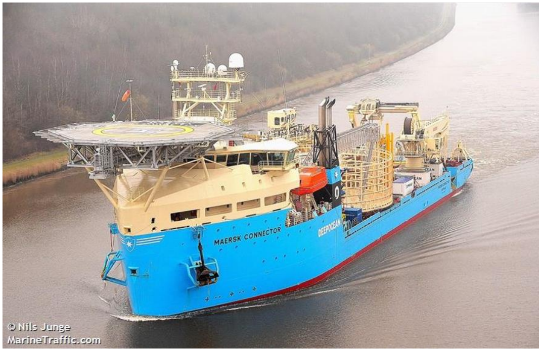
Figure 24. Rock Bag Placement and Boulder clearance vessel
