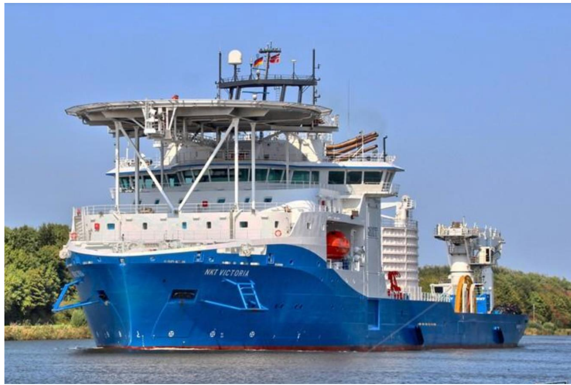
Figure 18. Cable lay vessel
