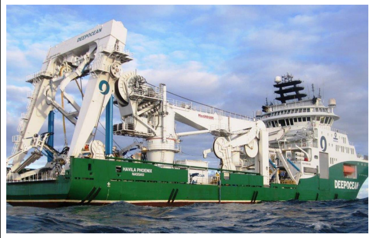
Figure 18. Cable burial vessel.
