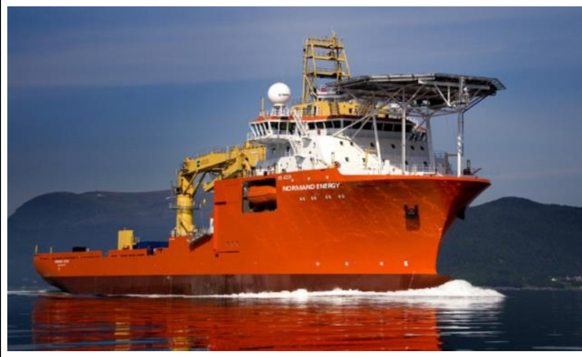
Figure 4. Soil Plug Removal Vessel
