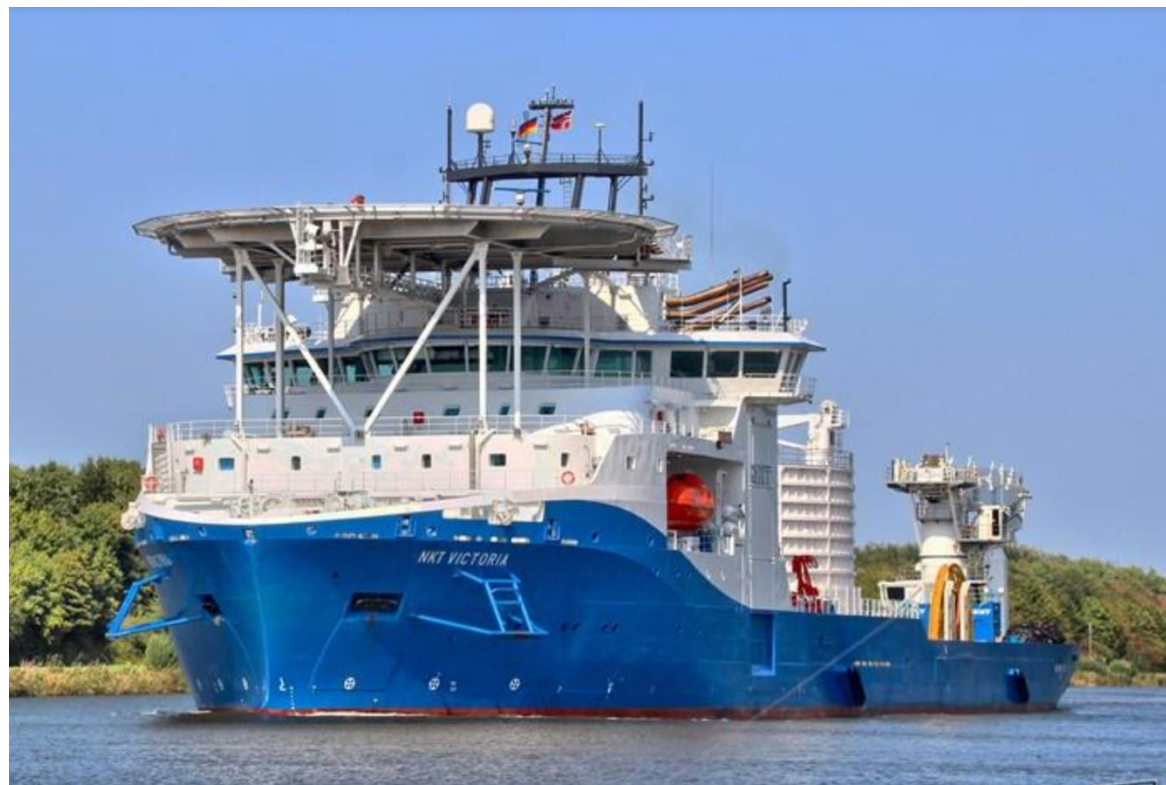
Figure 16. Cable lay vessel
