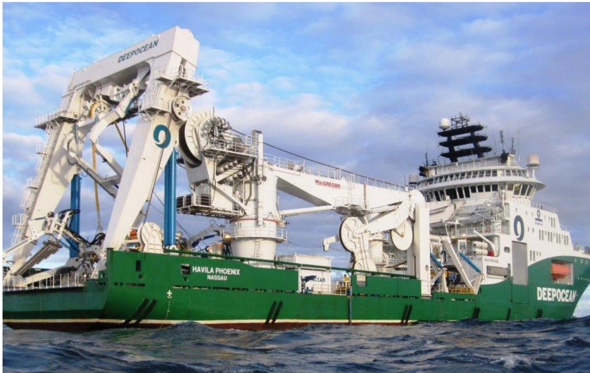
Figure 17. Cable burial vessel.
