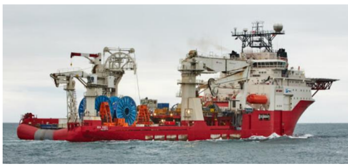
Figure 4 – Soil Plug Removal and Grouting Vessel
