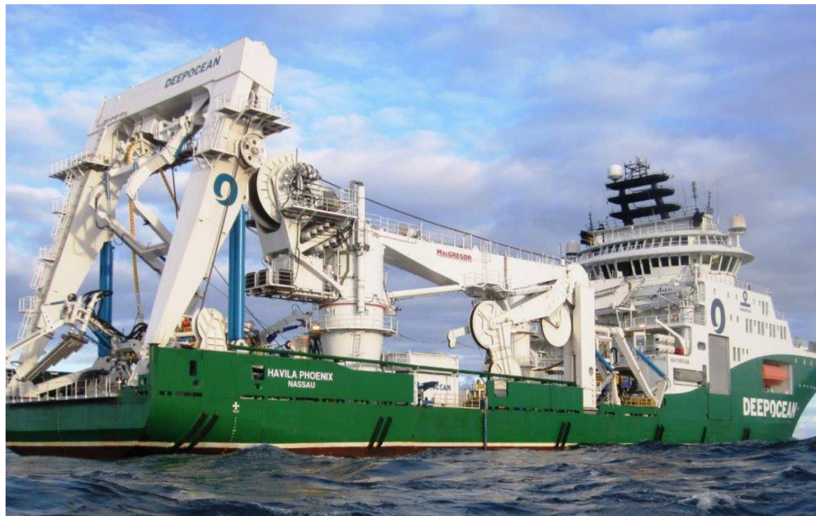
Figure 17. Cable burial vessel.
