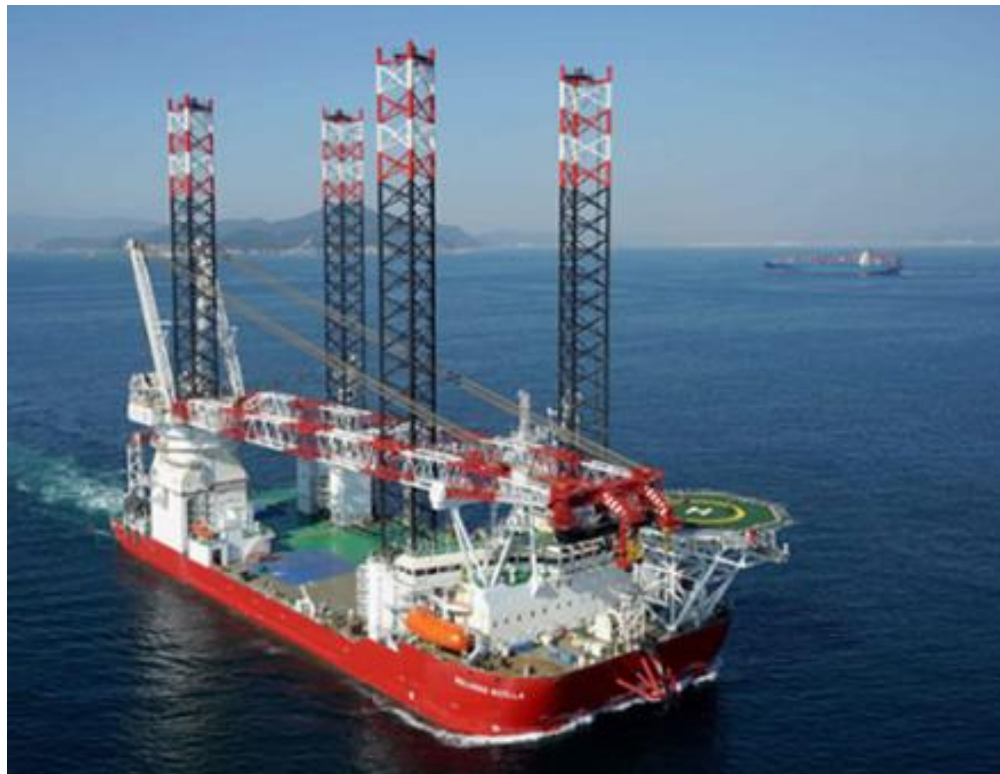
Figure 09. Jacket installation Vessel.
