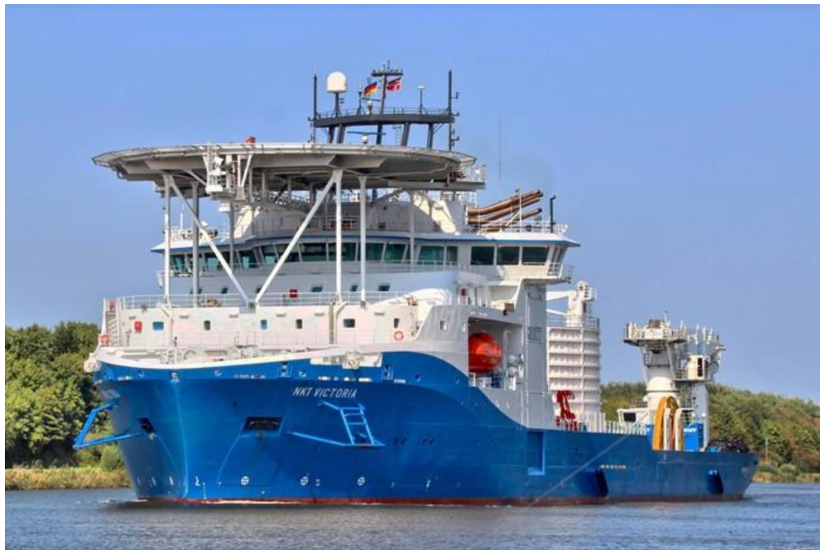
Figure 17. Cable lay vessel
