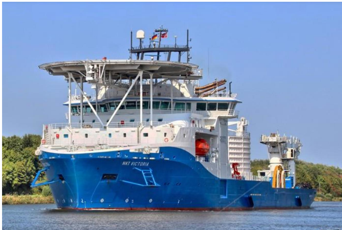
Figure 17. Cable lay vessel
