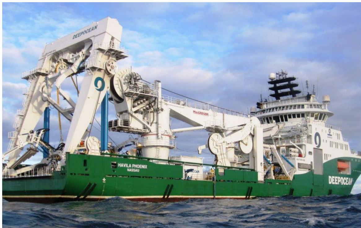
Figure 18. Cable burial vessel.
