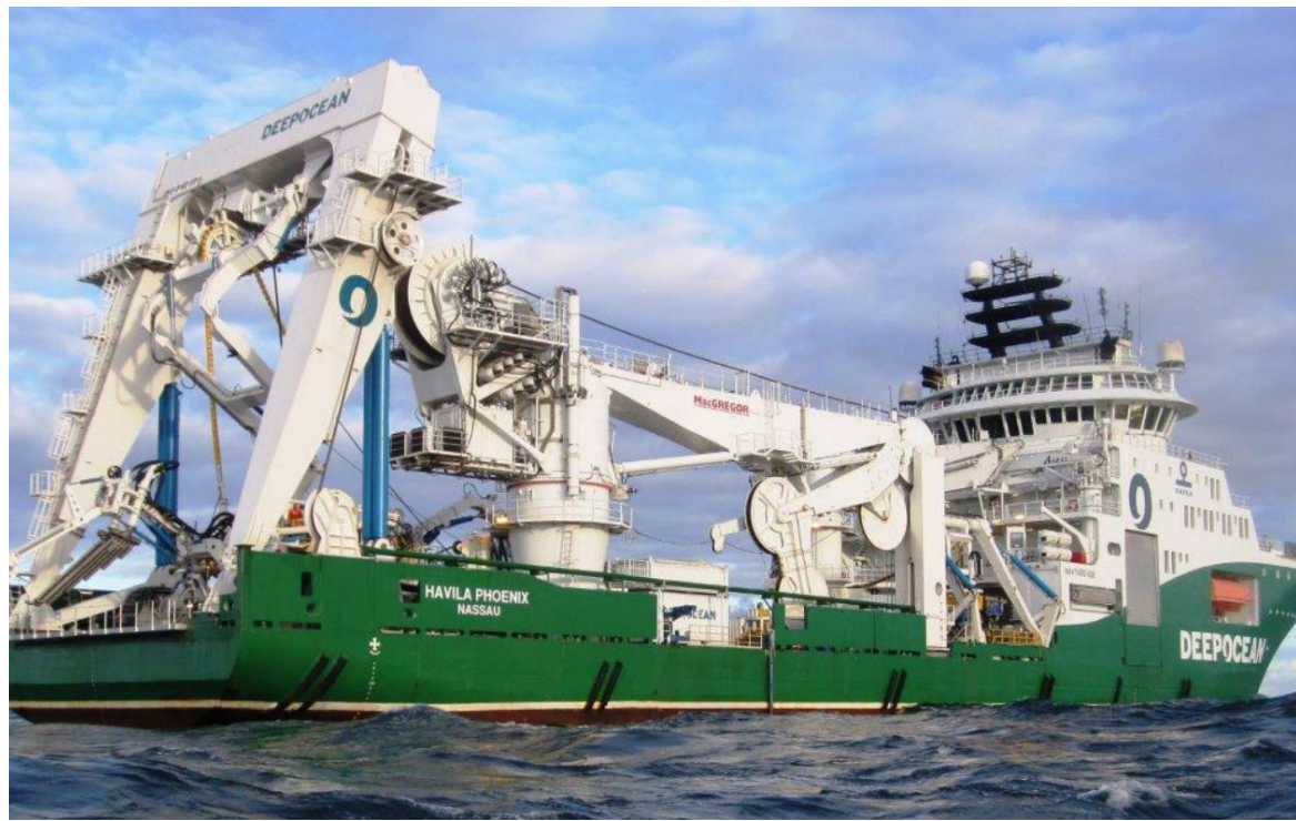
Figure 16. Cable burial vessel.
