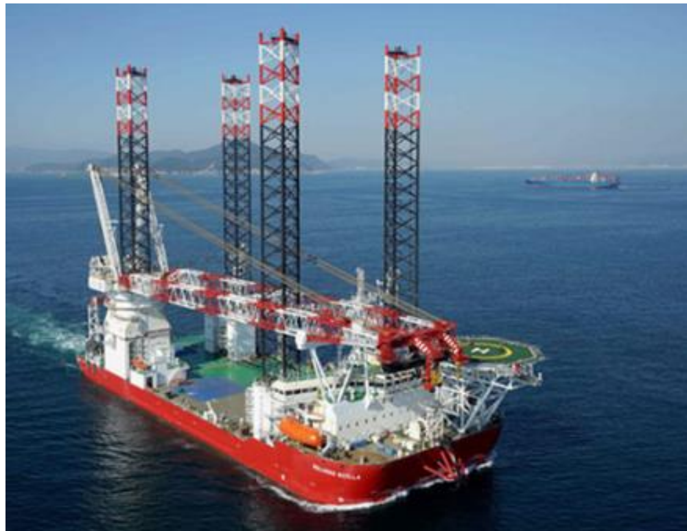
Figure 10. Jacket installation Vessel.
