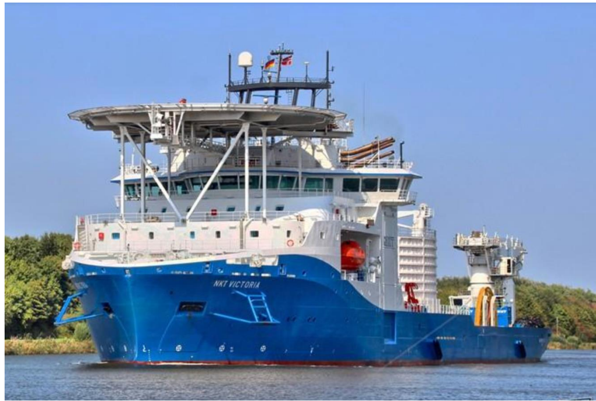
Figure 18. Cable lay vessel
