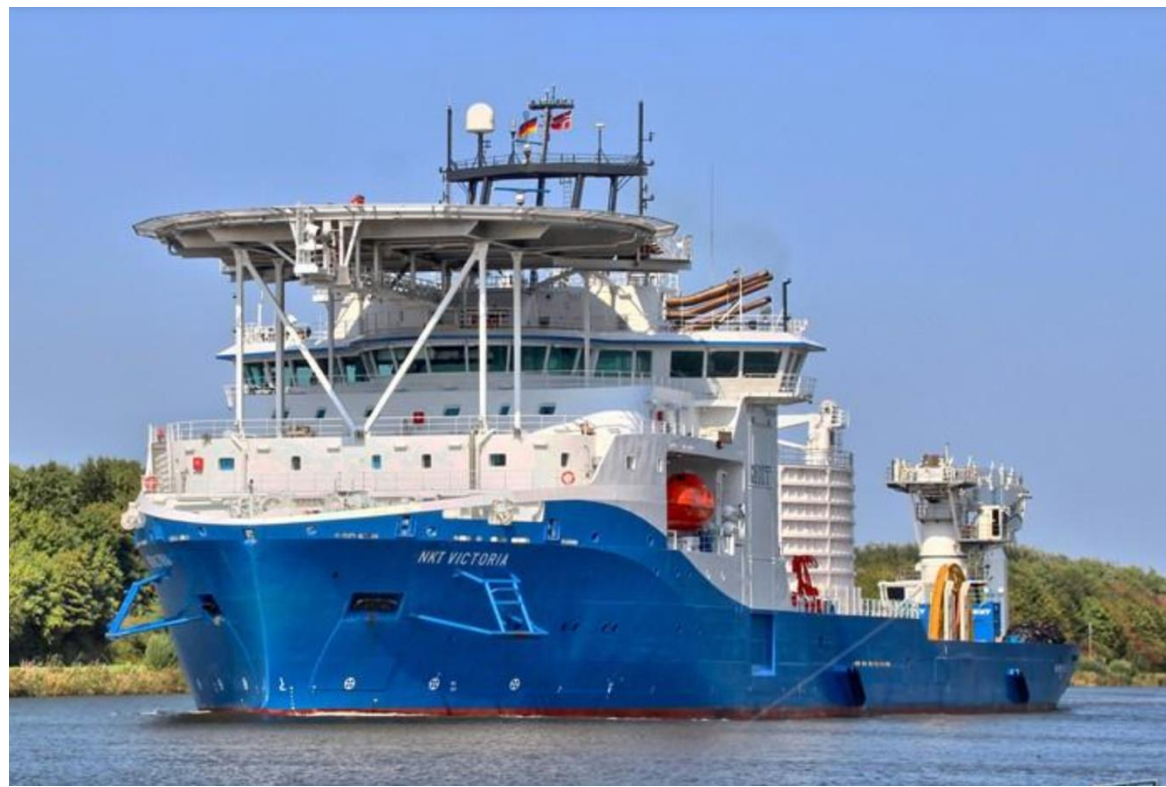
Figure 18. Cable lay vessel
