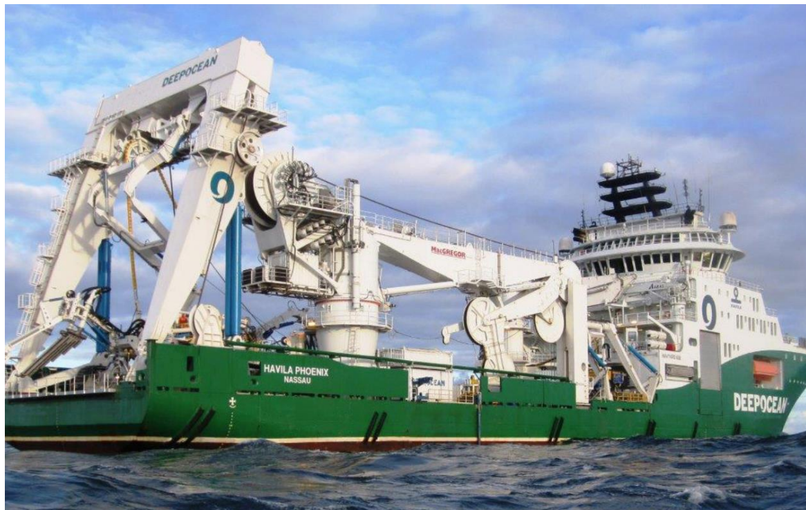
Figure 19. Cable burial vessel.
