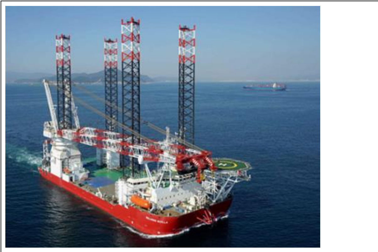
Figure 10. Jacket installation Vessel.
