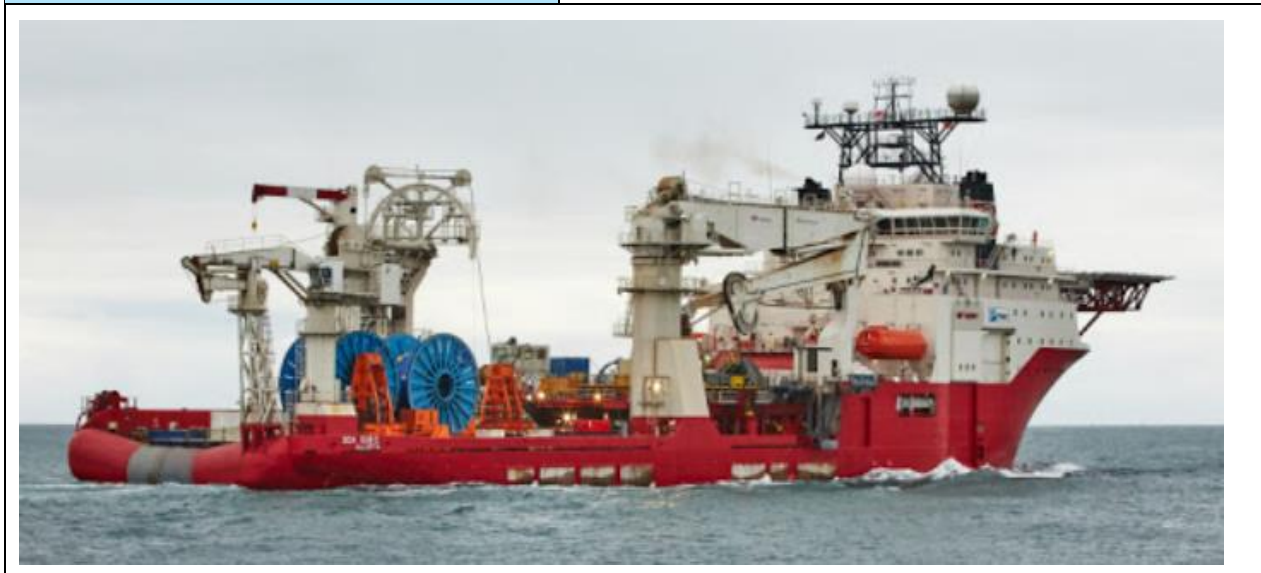
Figure 5 – Soil Plug Removal and Grouting Vessel
