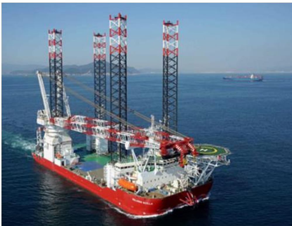
Figure 10. Jacket installation Vessel.
