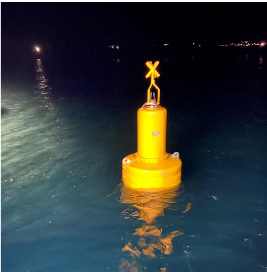
Figure 4 - Photograph of installed G1500 buoy
