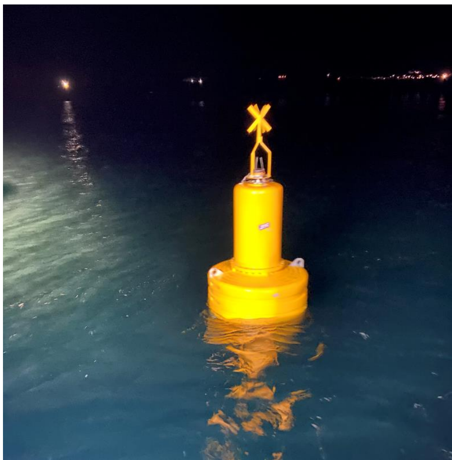
Figure 5 - Photograph of installed G1500 buoy
