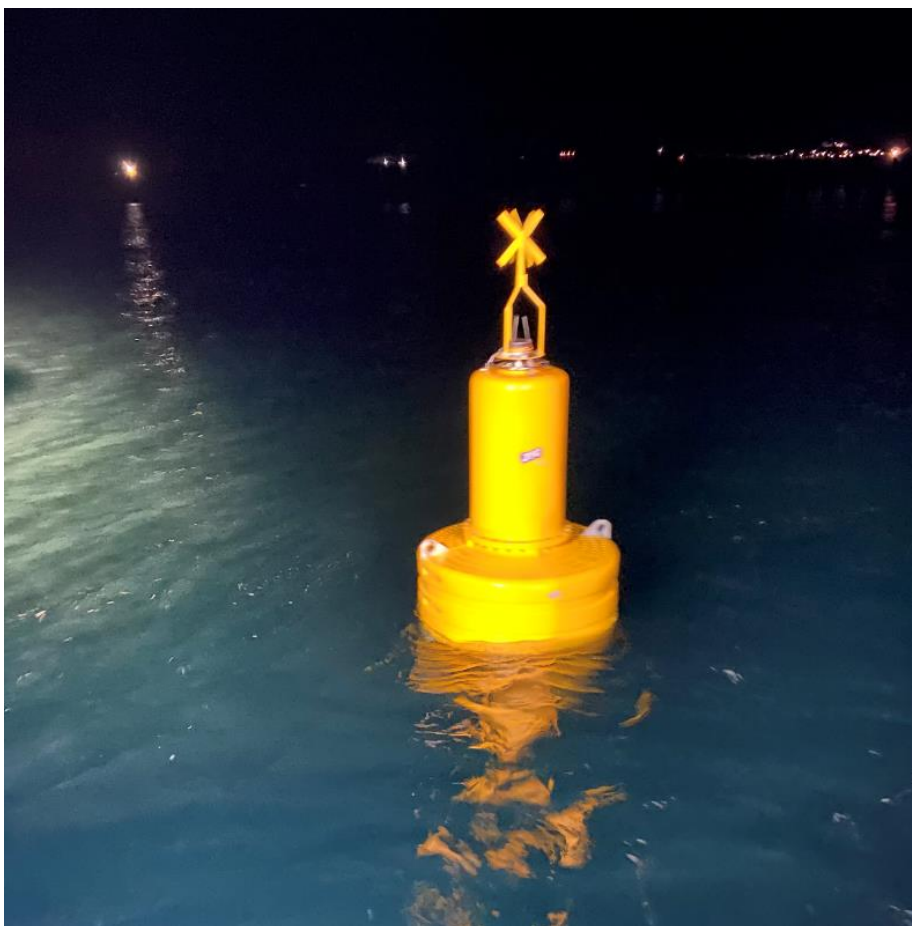
Figure 5 - Photograph of installed G1500 buoy
