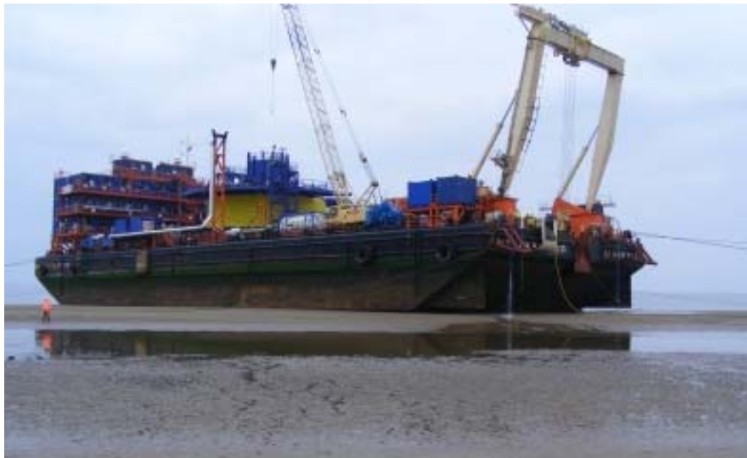
Figure 2-1: Cable lay barge aground
