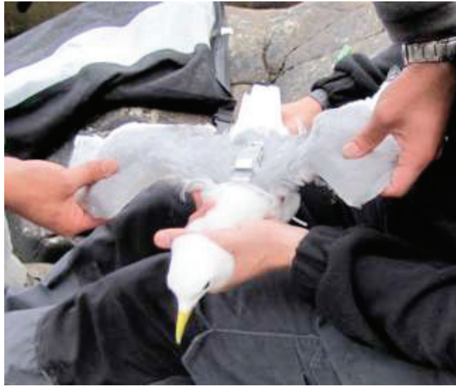
Fig. 2. Kittiwake fitted with an elastic harness to attach the GPS device. Excess elastic is visible in front of both wings; this was trimmed prior to release.
