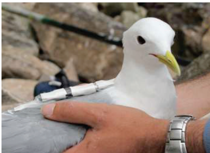
Fig. 3. Kittiwake fitted with an elongated GPS logger attached using white Tesa tape.
